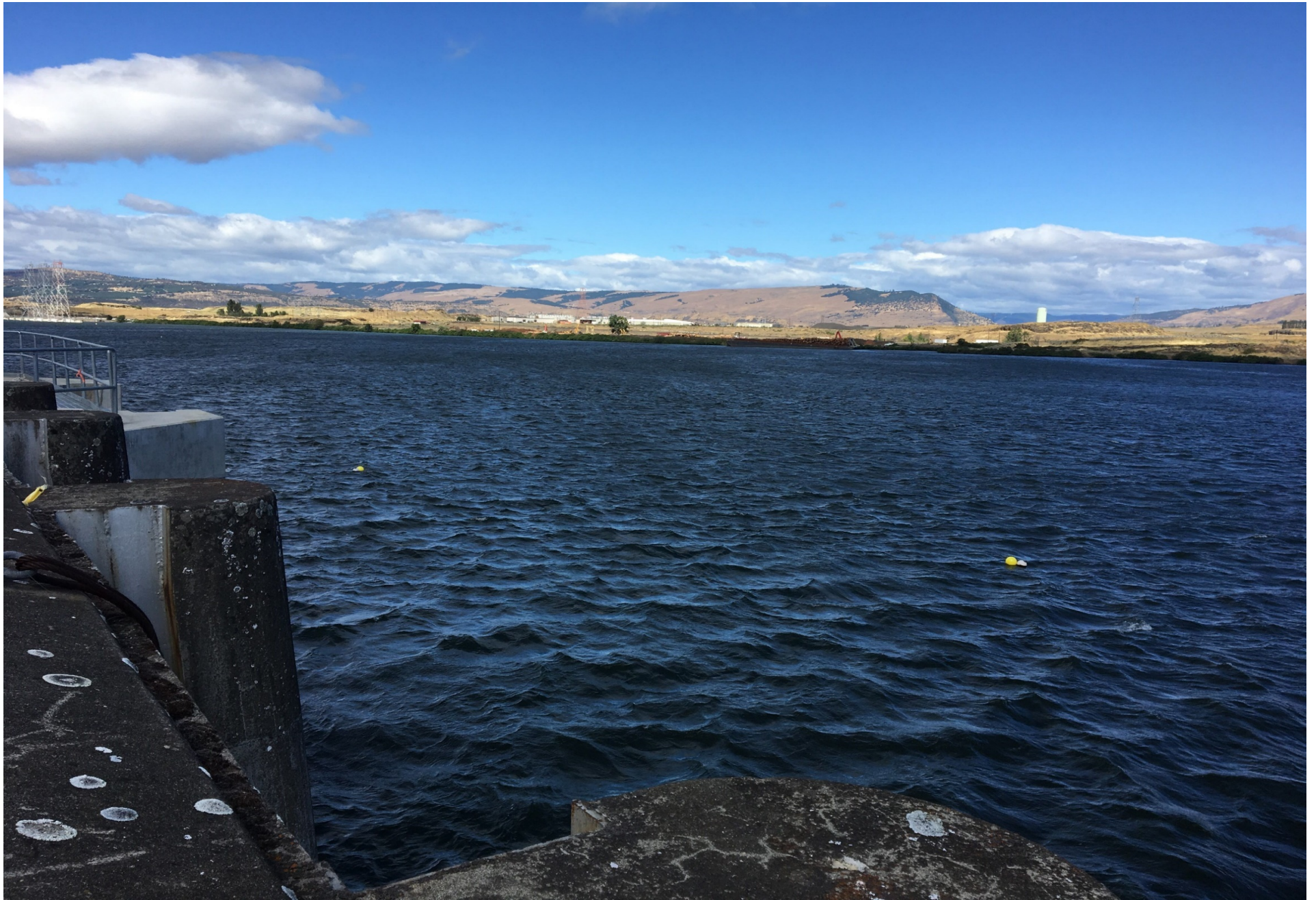
Floating temperature profile strings in the BRZ-East Exit Temperature profile data to be analyzed for thermal stratification
